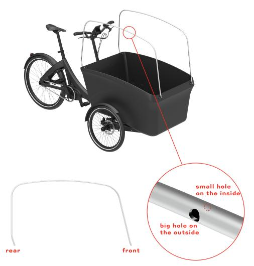
**4-** Take the 2 side frame tubes and insert them into the front and rear brackets pins. The big holes have to point to the outside.
