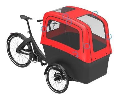
**7-** Take the 8 turn locks and mount them on the prepared positions, shown by the red circles, using 2x M4.2x13 screws on each lock. Use 3 Nm (2,21 ft-lb) force.
