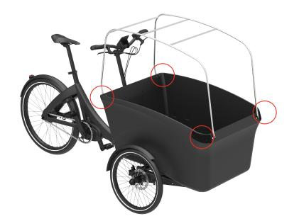
**5**- Take the 2 (2 kids hood) or 3 (4 kids hood) short straight bars and fix them to the side frame tubes with the DIN912 M4x14 screws.
